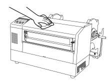
5.1.3 Optional Cutter Module 1. Remove the Plastic Head Screws and to detach the Cutter Cover.
